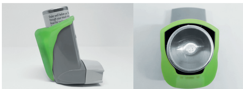
Figure 7. 3D-printed inhaler clip-on containing the Sensirion flow sensor SDP3x in the side view (left) and top view (right) showing the unobstructed flow path of the inhaler.
