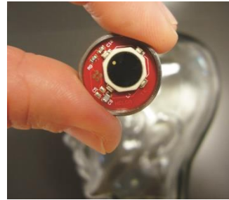
Micro Implant for long-term intracranial pressure monitoring.
