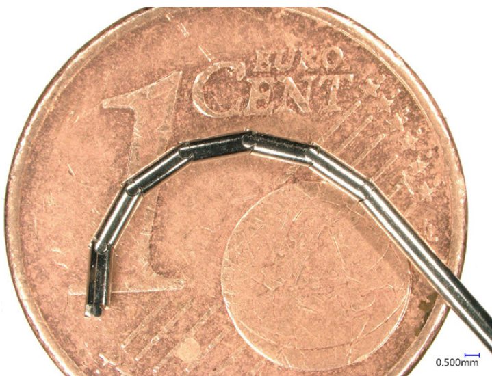
Laser machined SST capillary Ø0,9mm Source: Veldlaser
