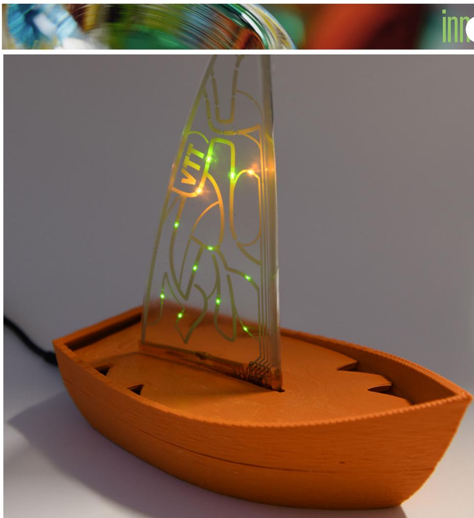
Bio-polymer based structural electronics demonstrator (CO<sub>2</sub> sensor), Source: VTT
