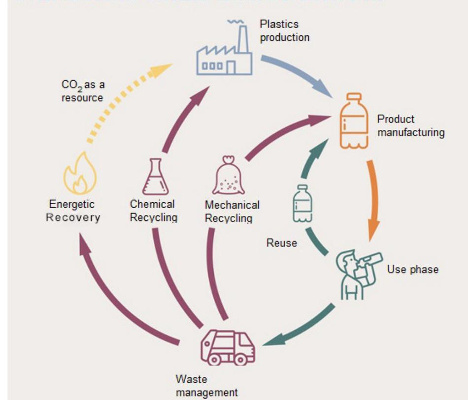
A German overview of a possible plastic cycle: from production through product manufacturing, use phase and recycling or waste management with subsequent energy recovery (with the use of CO<sub>2</sub> as a raw material), chemical recycling or mechanical recycling.
